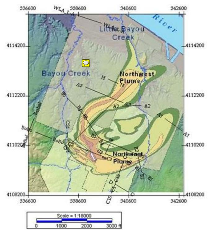
**Exhibit 8.** A map shows the contamination plume migration paths according to groundwater samples analysis of intense boreholes distribution across the plume. Modified from (Blits, 2008).
