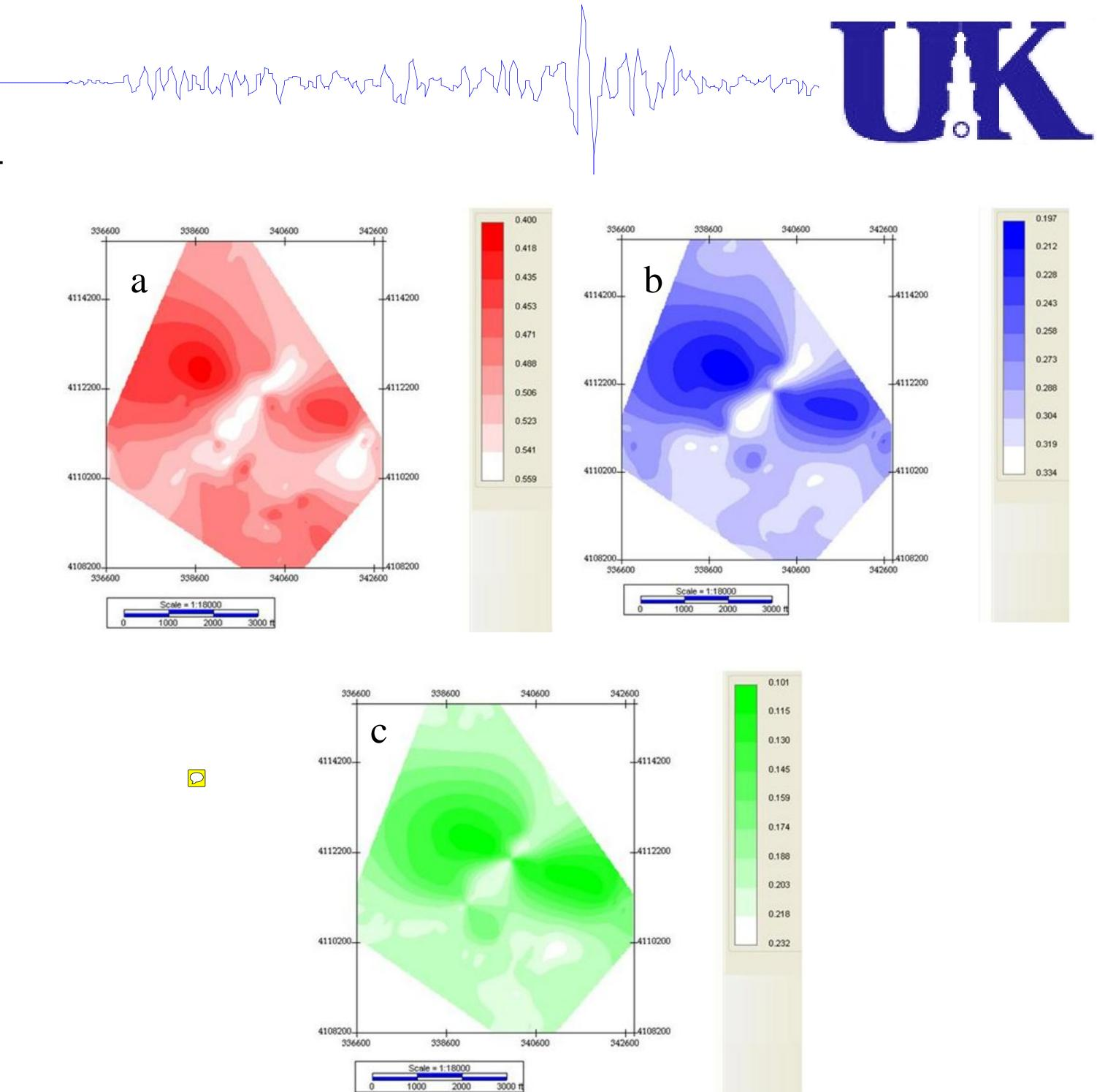
**Exhibit 7.** Isochronal maps, **a**) the red-fill contours are Paleozoic bedrock, **b**) the bluefilled contours are the Cretaceous McNairy, c) and the green-filled contours are the Pleistocene Mound Gravel aquifer. As it is noticeable in all isochronal maps, the the white areas correspond to the deepest places due to the faults offsets. Specifically, the faults trends control the migration of a contamination plume toward northeast direction in the Mound Gravel Aquifer.
