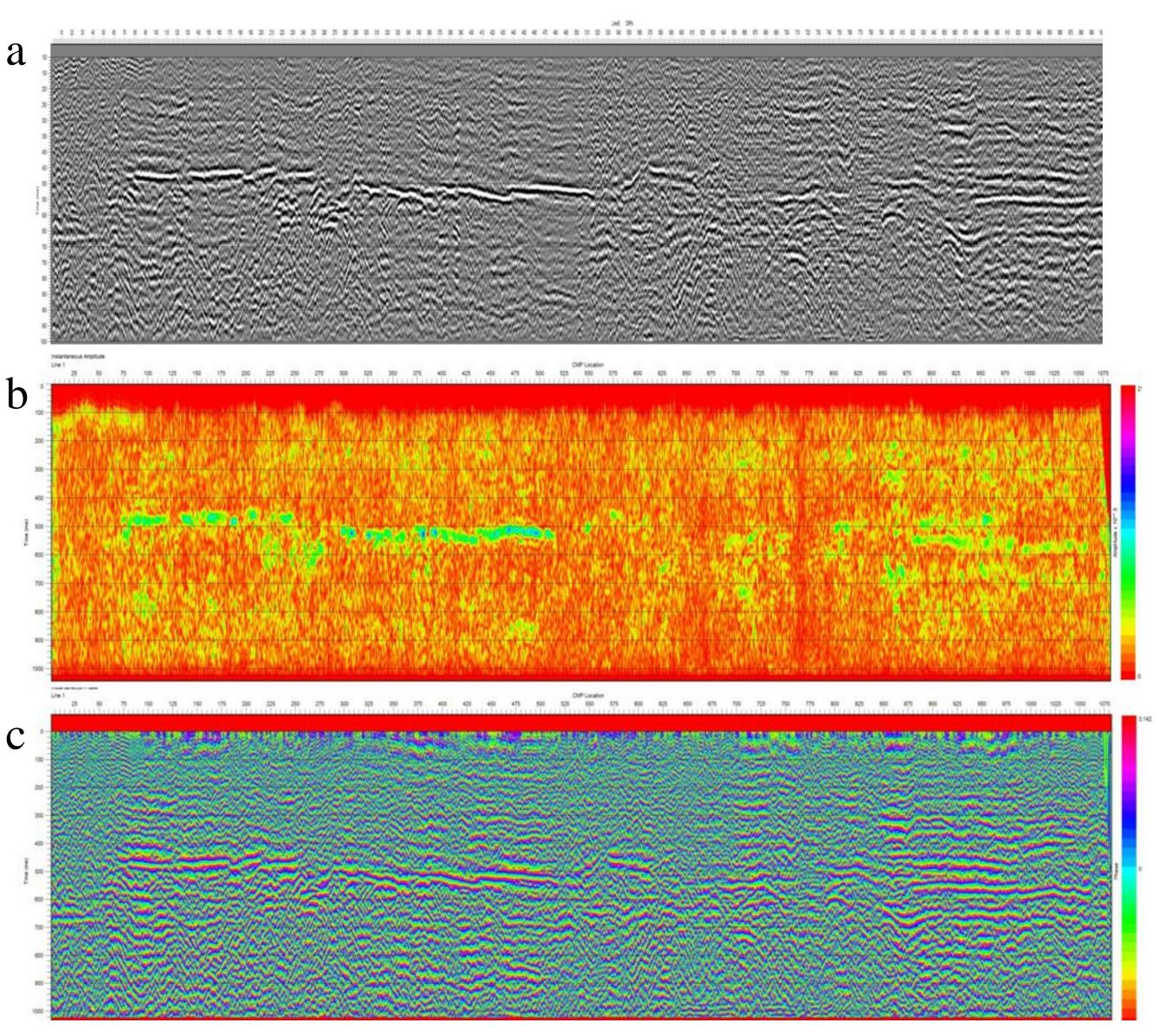
Exhibit 4. a) Final stack seismic profile of line-B, E-W. The conventional seismic data processing procedure was applied using Seismic data Processing Workshop package (SPW 2.1.20). b) Post stack instantaneous amplitude section of the same seismic profile. c) Post stack instantaneous phase section of the seismic profile. Note, the same seismic data processing procedure was applied to all seismic profiles, and this profile is an example of final stack and post stack processing.
