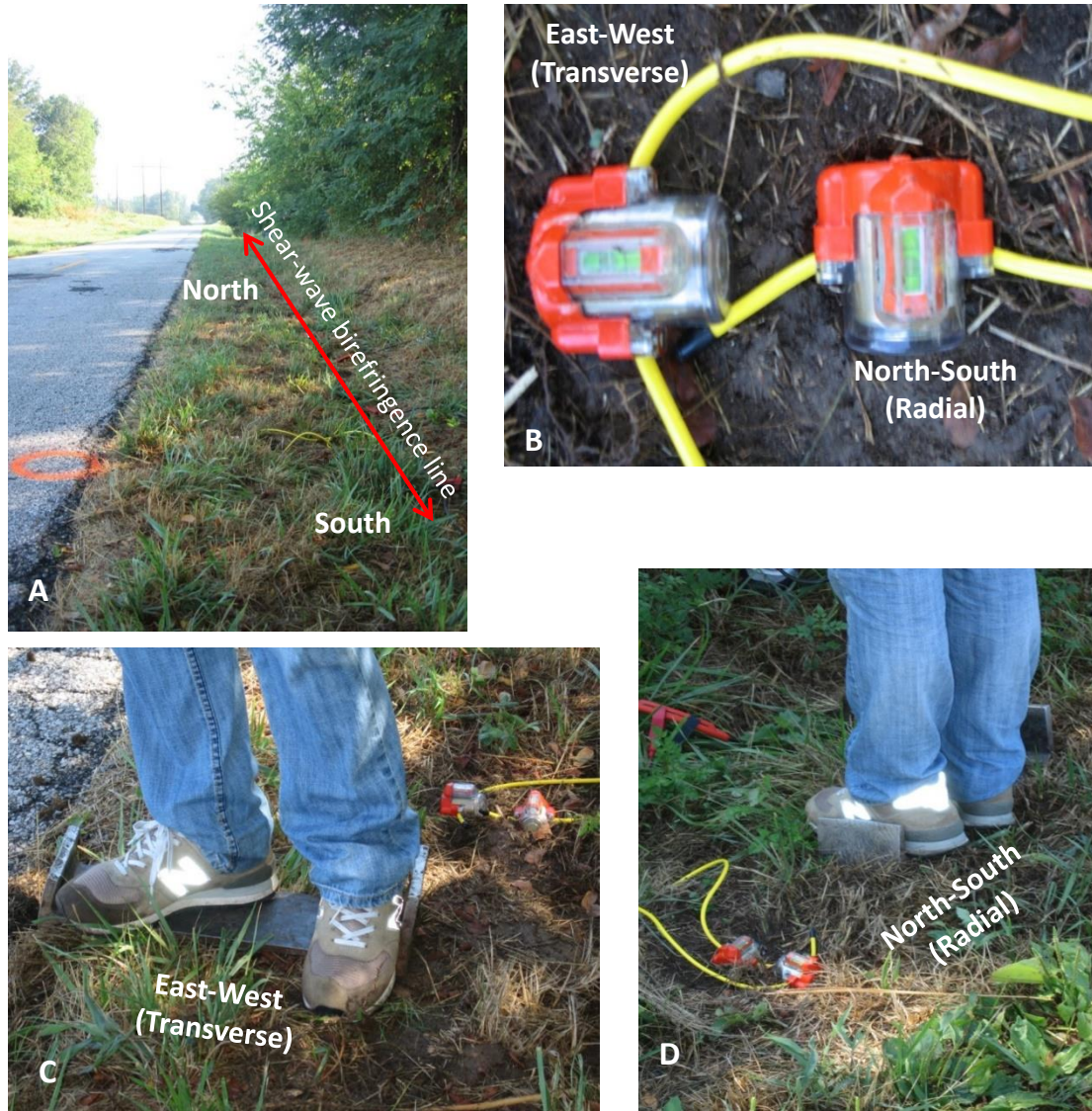
Figure 2.7: (A) Shear-wave splitting line direction. (B) A pair of two single-component horizontal-polarization 30-Hz geophones aligned perpendicular ( 90^\circ ) to each other. (C) East-west SH-wave source in-line with east-west geophone and perpendicular with the north-south geophone. (D) North-south SH-wave source in-line with north-south geophone and perpendicular with the east-west geophone.
