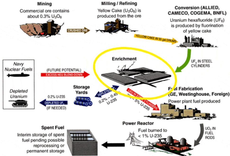
Figure 1.2.2 The Uranium Fuel Cycle (US DOE, 2011b)
