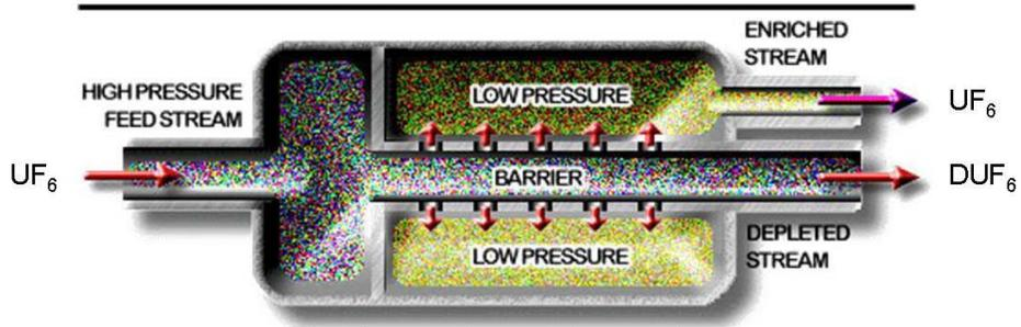
This process of uranium enrichment increases the concentration of U-235 from 0.7% up to 5.0%
